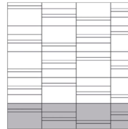
SCHEMA 10 11%/mq 5x60 cm 22%/mq 10x60 cm 33%/mq 15x60 cm 33%/mq 30x60 cm
